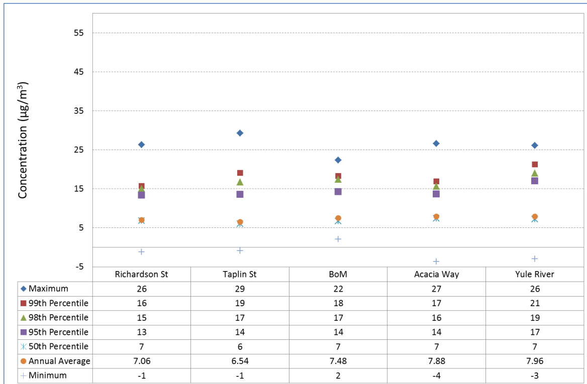
Figure B-1: Statistical summary of 24-hour and annual averages of PM 2.5 concentration in FY14
