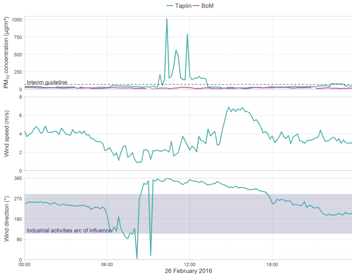
Figure 7-18: Time series of PM 10 concentrations at Taplin and BoM (top) and Taplin wind speed (middle) and wind direction (bottom) on 26 February 2016
