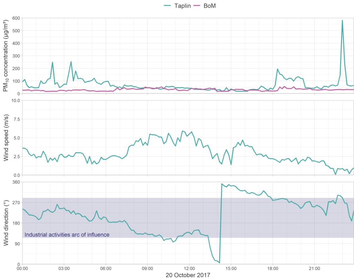
Figure 8-3: Time series of concentrations of PM 10 at Taplin and BoM (top) and wind speed at Taplin (middle) and wind direction at Taplin (bottom) on 20 October 2017
