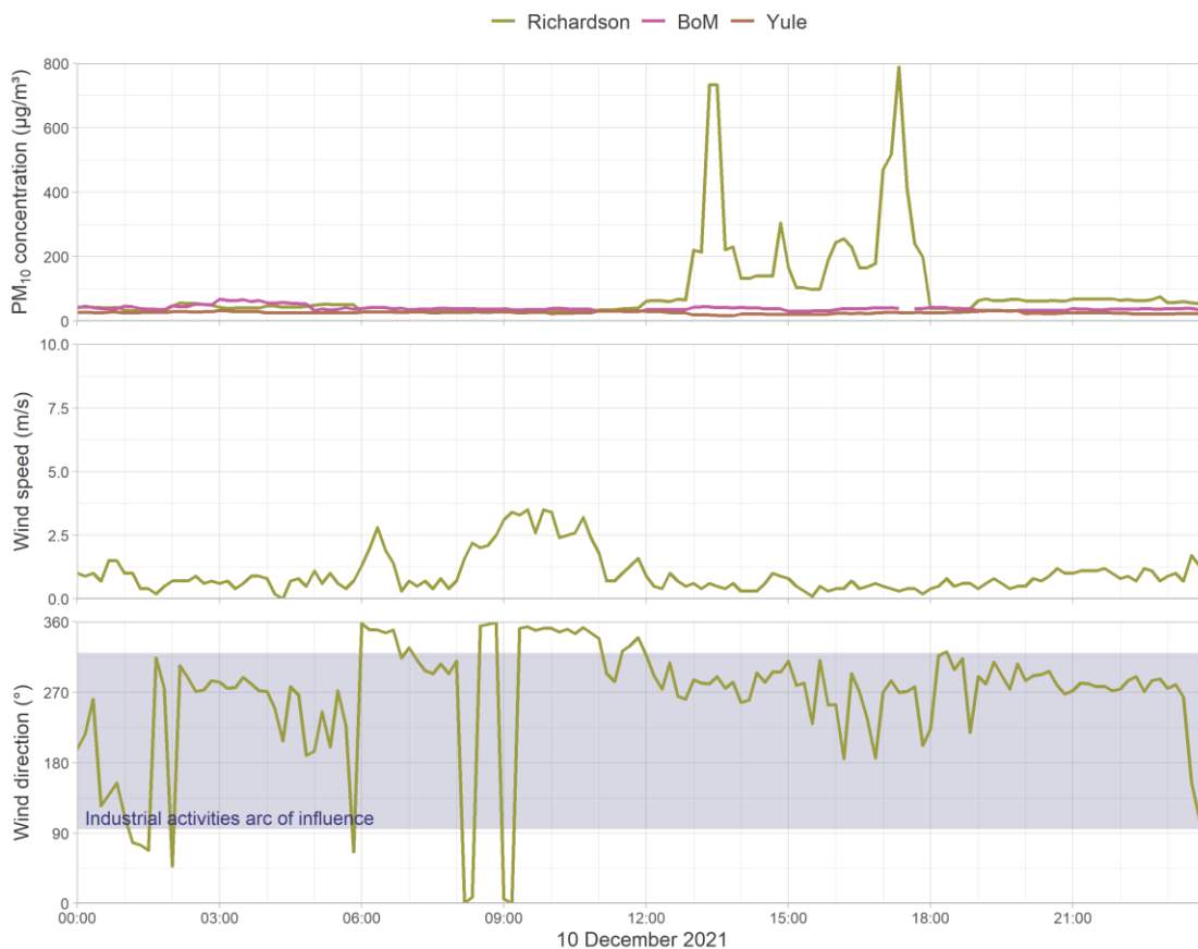
Figure 10-14: Time series of concentrations of PM 10 at Richardson, BoM and Yule (top) and wind speed at Richardson (middle) and wind direction at Richardson (bottom) on 10 December 2021
