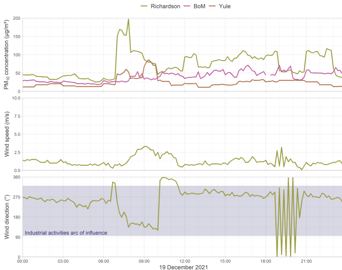
Figure 10-18: Time series of concentrations of PM 10 at Richardson, BoM, and Yule (top) and wind speed at Richardson (middle) and wind direction at Richardson (bottom) on 19 December 2021
