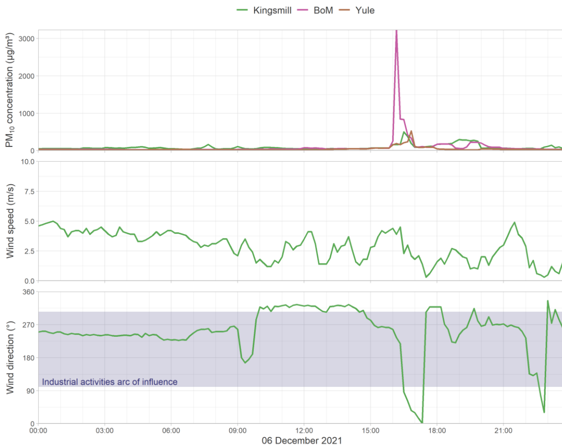
Figure 10-12: Time series of concentrations of PM 10 at Kingsmill, BoM, and Yule (top) and wind speed at Kingsmill (middle) and wind direction at Kingsmill (bottom) on 6 December 2021
