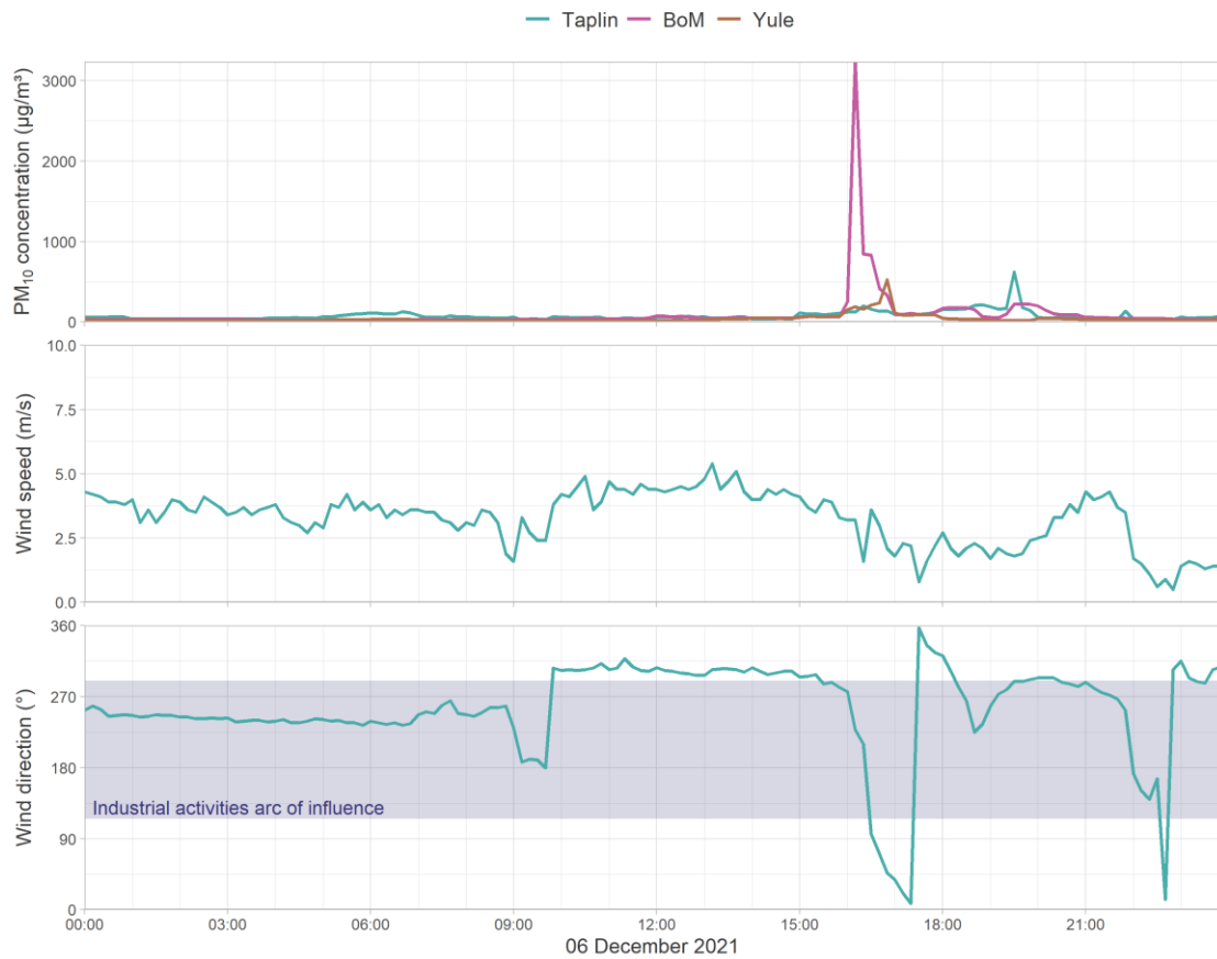
Figure 7-12: Time series of concentrations of PM 10 at Taplin, BoM, and Yule (top) and wind speed at Taplin (middle) and wind direction at Taplin (bottom) on 6 December 2021
