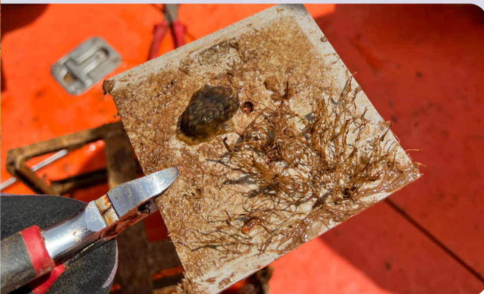
Marine growth on an array.
